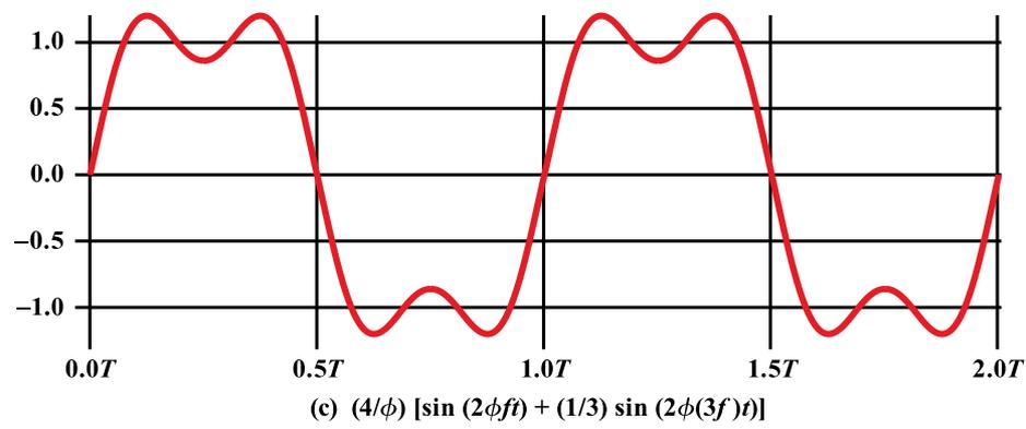
**Addition of frequency Components ( $T = 1/f$ )**
